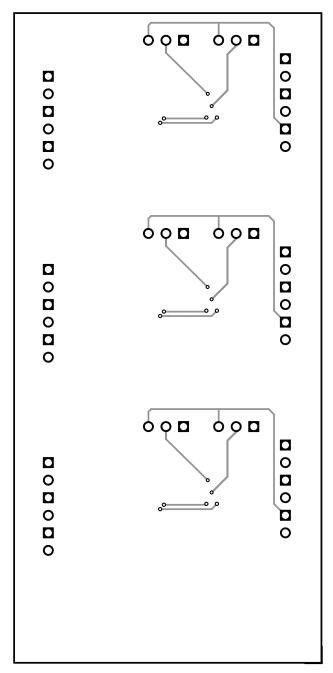
Figure 3. Bottom Layer Routing
