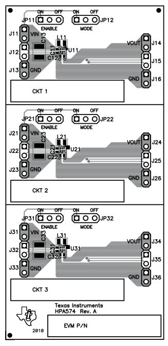
Figure 1. Assembly Layer
