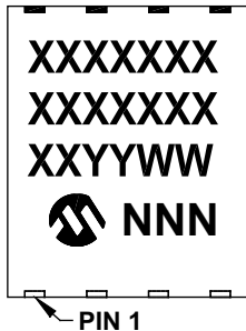
8-Lead PDFN (5x6x1.0 mm)
