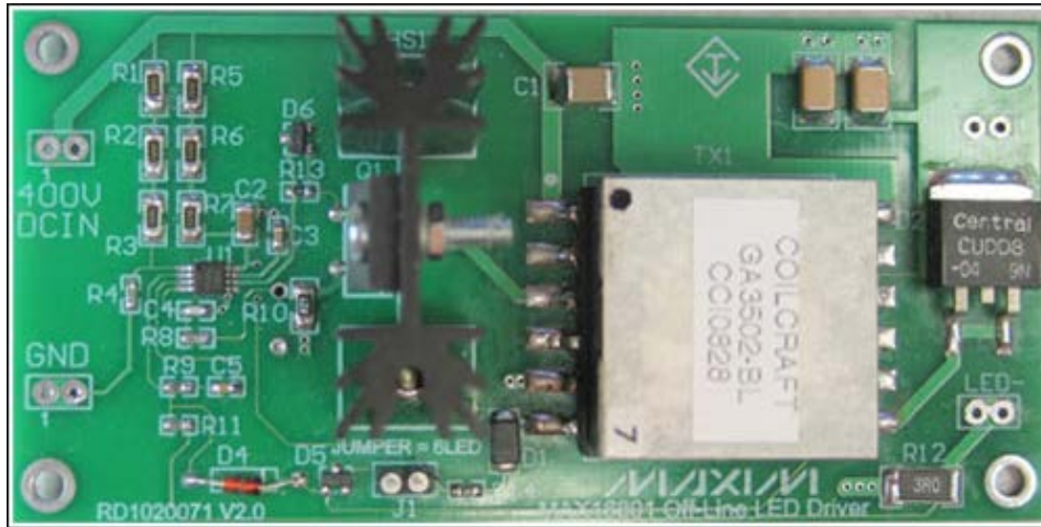
Figure 1. The LED driver reference design is 1.9in x 3.9in, double sided.
