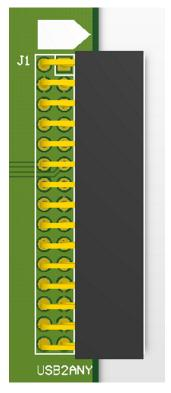
Figure 2-4. USB2ANY Interface Connector
