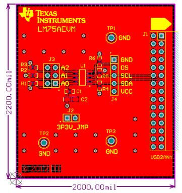
Figure 5-1. Top Assembly Layer
