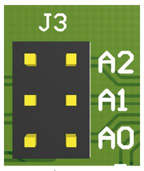
Figure 2-5. I<sup>2</sup>C Slave Select Jumper
