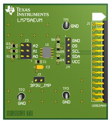
Figure 2-1. LM75A Evaluation Board
