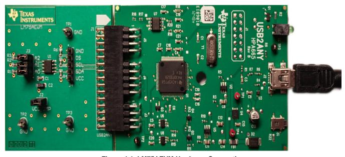
Figure 4-1. LM75AEVM Hardware Connection
