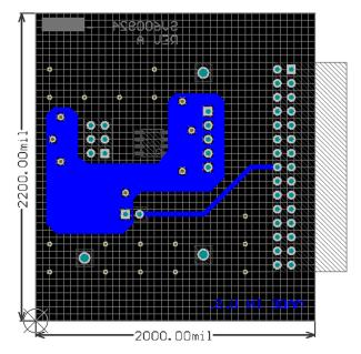
Figure 5-3. Bottom Layer Routing
