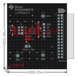
Figure 5-2. Top Layer Routing
