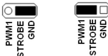
Figure 3. STROBE Jumper Settings
