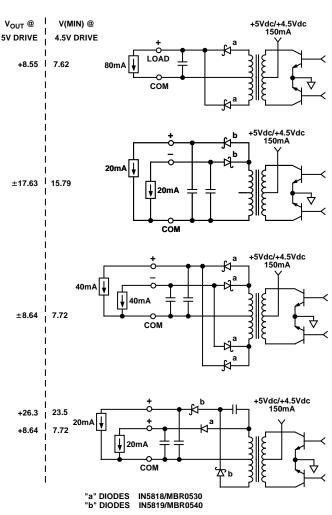
Figure 5. Field Side Power Supply Rectifier Examples
