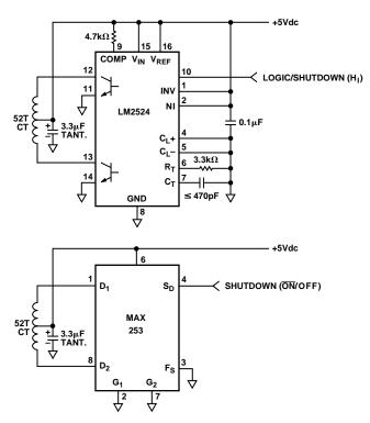
Figure 3. System Side Transformer Driver Examples
