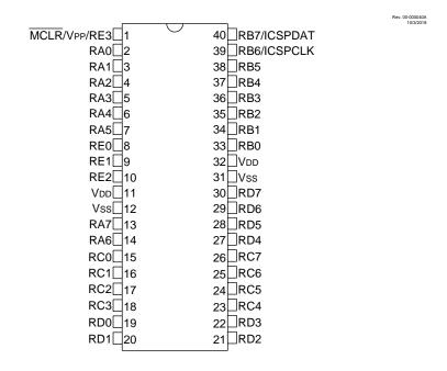
Figure 4. 40-pin QFN
