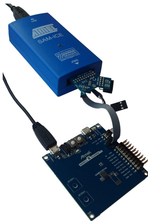
Figure 7-2. SAM-ICE using an Atmel-ICE Adapter
