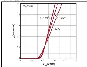
FIGURE 2-8: Transfer Characteristics.
