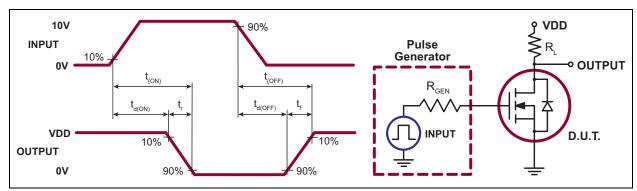
FIGURE 4-1: Switching Waveforms and Test Circuit.
