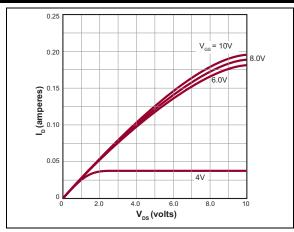
FIGURE 2-4: Saturation Characteristics.
