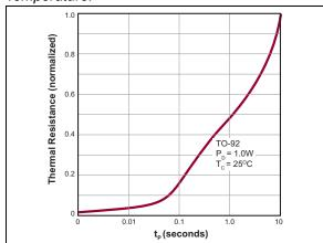
**FIGURE 2-6:** Thermal Response Characteristics.
