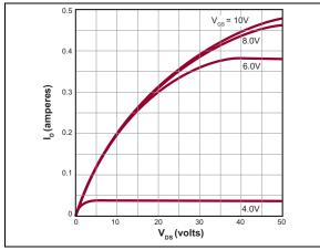
FIGURE 2-1: Output Characteristics.
