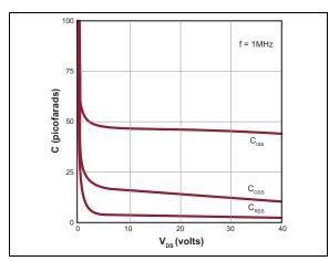
FIGURE 2-9: Capacitance vs. Drain-to-Source Voltage.
