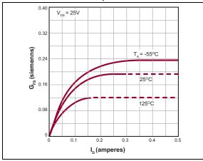
**FIGURE 2-2:** Transconductance vs. Drain Current.
