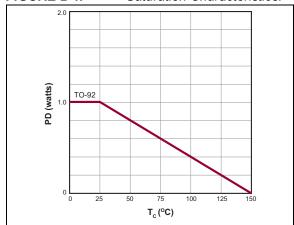
**FIGURE 2-5:** Power Dissipation vs. Case Temperature.
