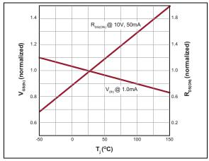
V<sub>(th)</sub> and R<sub>DS</sub> Variation with **FIGURE 2-11:** Temperature.
