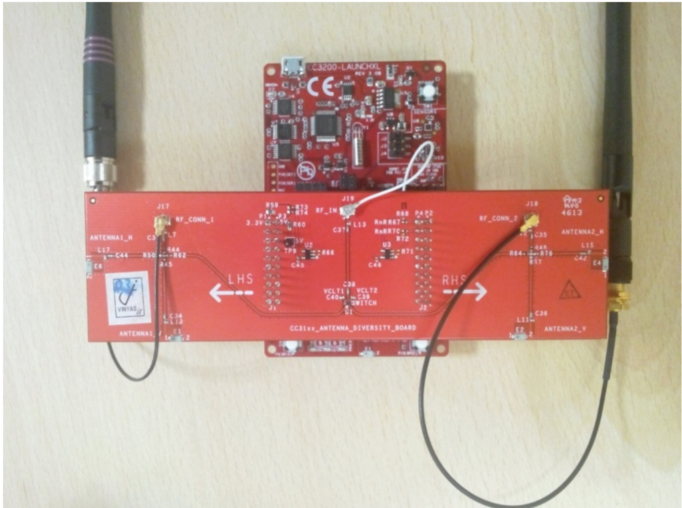
Figure 3-3. Correctly Connected CC3200-LAUNCHXL and CC3ANTENNABOOST Boards
