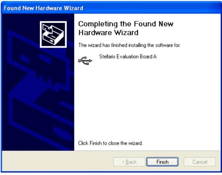
You have just installed the drivers for "Stellaris Evaluation Board A." The USB device built into the EVB is a composite USB device. After you click Finish, Windows automatically installs a driver for the "Stellaris Evaluation Board B" part of the composite USB device. Follow the same instructions as above to install the drivers for this device.
