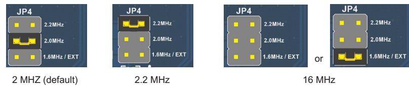
Figure 6. Switching Frequency Jumper Settings
