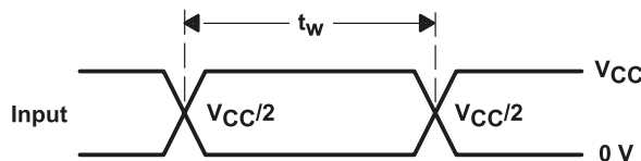
Figure 2. Voltage Waveforms Pulse Duration
