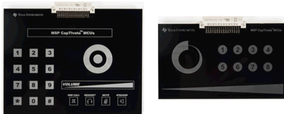
Figure 7-6. CAPTIVATE-PHONE and CAPTIVATE-BSWP Panels
