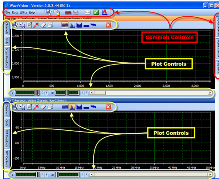
Figure 6. WaveVision 5 overview of control buttons
