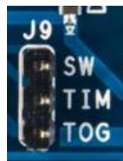
Fig 2. Selection of operating mode using jumper J9
