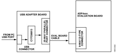
Figure 2. USB Adapter Board Setup
