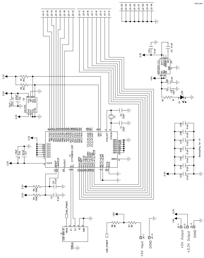
Figure 3. Evaluation Board Schematic
