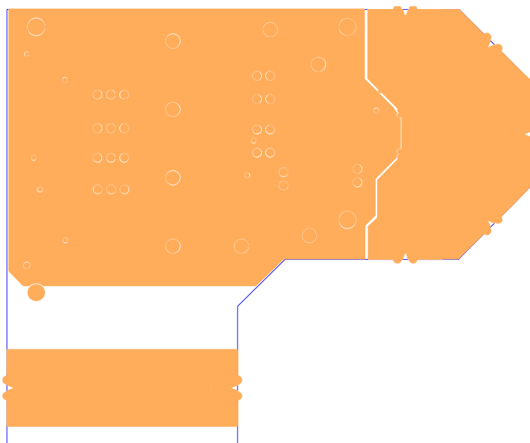
Figure 14. EVAL-ADGM1304SDZ Component Side Ground Plane PCB Drawing (Layer 2)
