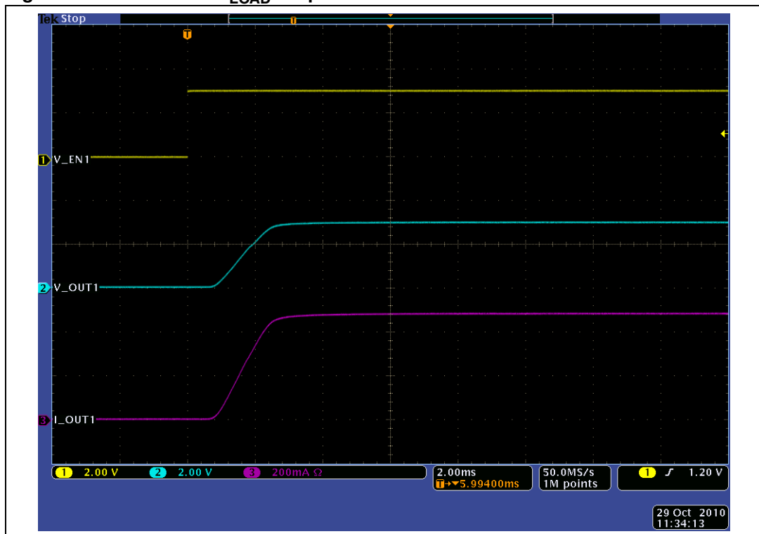
Figure 3. Turn-on for C_{\text{LOAD}} = 1\ \mu\text{F}
