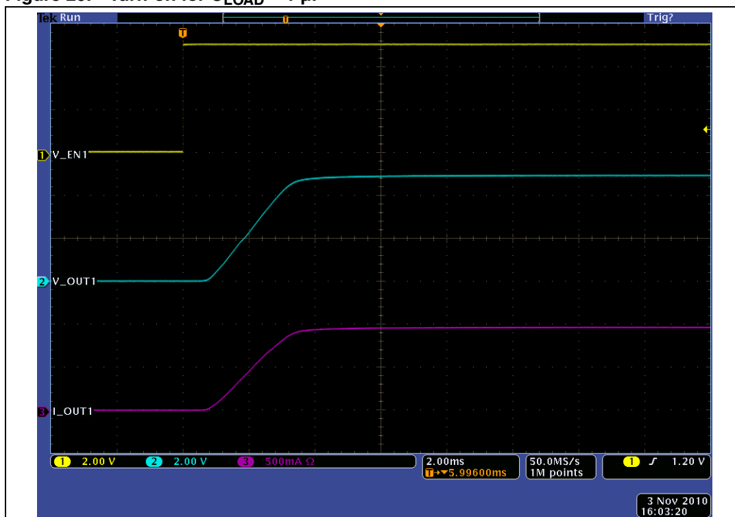
Figure 29. Turn-on for C_{LOAD} = 1 \mu F
