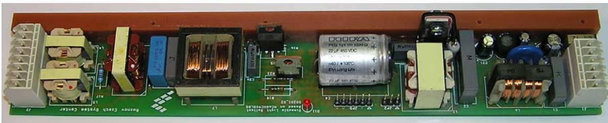
Figure 4-1. Dimmable Light Ballast - Demo Board
