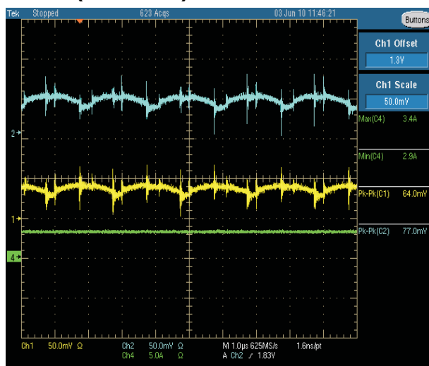
Figure 10. Ripple for Buck 1 (Yellow Trace) 1.2 V, 3 A and Buck 2 (Blue Trace) 1.8 V, 2 A, 50 mV per Division V_{IN} = 12\text{ V} , f_{SW} = 500\text{ kHz} , L_O = 4.7\text{ }\mu\text{H} , DCR = 10 m \Omega , C_O = 22\text{ }\mu\text{F}
