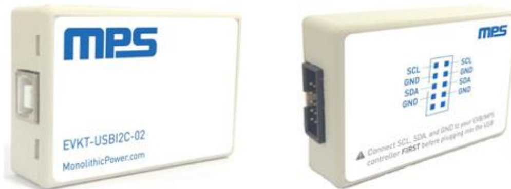
Figure 3: EVKT-USBI2C-02 Communication Interface
