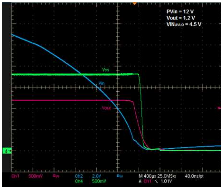
Figure 5. UVLO Shutdown Waveform
