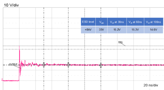
Figure 7: ESD response to IEC 61000-4-2 (+8kV contact discharge)
