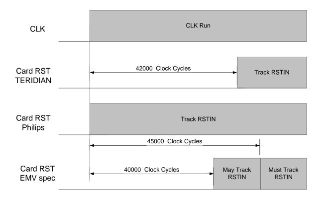
Once card RST is de-asserted, the system controller expects an ATR response from the card within a certain window of time. If the ATR is not properly received before the end of this window an ATR timeout error will occur.
