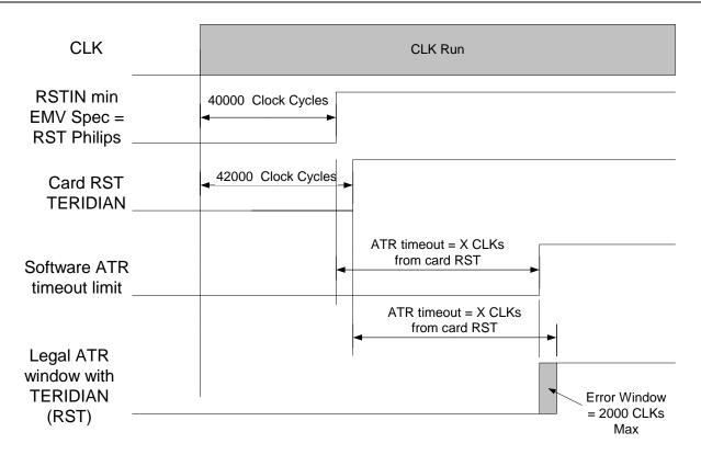
Due to the timing difference between the devices in the case of RSTIN being de-asserted between 40000 and 42000 clock cycles after CLK, there is a delay between RSTIN and card RST up to 2000 clock cycles. This means that a card can respond with a valid ATR response (with respect to card RST) and still generate an ATR timeout error (with respect to RSTIN)
