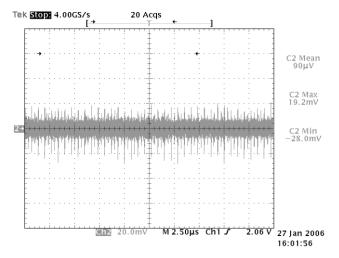
Figure 5: Teridian 73S8024RN, GND (Pin 22)
