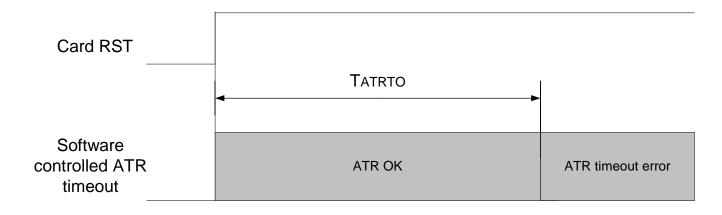
With the TDA8024T, this timeout starts at the rising edge of RSTIN. If the system controller de-asserts RSTIN between 40000 and 42000 clock cycles after CLK starts, the card RST signal timing will be different between the TDA8024T and the Teridian 8024RN.
