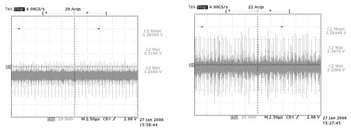
Figure 9: 73S8024RN V<sub>DD</sub> Digital Power Supply (Pin 21) Figure 10: TDA8024T, V<sub>DD</sub> Digital Power Supply (Pin 21)
