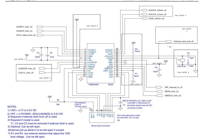
Figure 11: Teridian 73S8024RN Application Schematic
