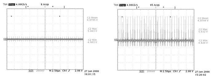
Figure 7: 73S8024RN V<sub>PC</sub>, Regulator Supply (Pin 6) Figure 8: TDA8024T V<sub>DDP</sub>, DC/DC Converter Power Supply (Pin 6)
