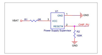
Figure 6: Reset Circuit
