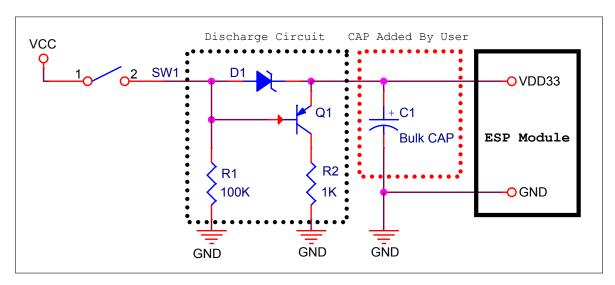
Figure 5: Discharge Circuit for VDD33 Rail
