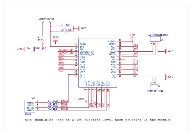
Figure 4: ESP32-SOLO-1 Peripheral Schematics
