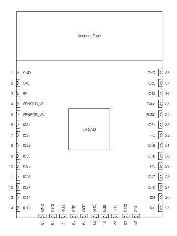
Figure 1: ESP32-SOLO-1 Pin Layout (Top View)
