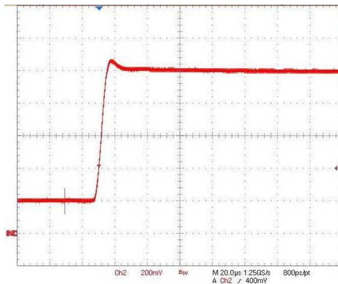
Figure 75. Loop Current Step From 4 mA to 20 mA
