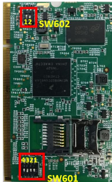
Fig 16. i.MX6UltraLite (MCIMX6UL-EVKB) board switches
