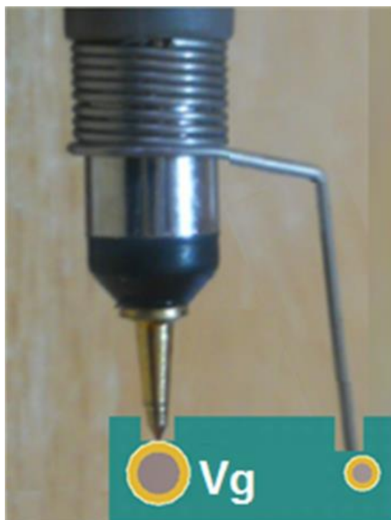
Figure 6. Recommended Use for Ground Spring Clip Test Points
