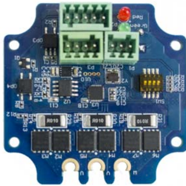
Motor Control PCBA
