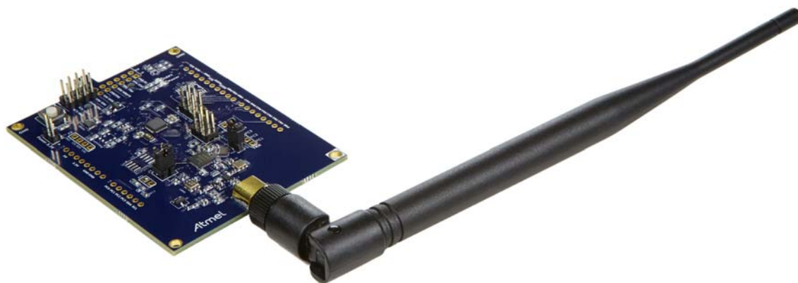
Figure 1-2. ATA8520-EK3-E Xplained Pro Extension
