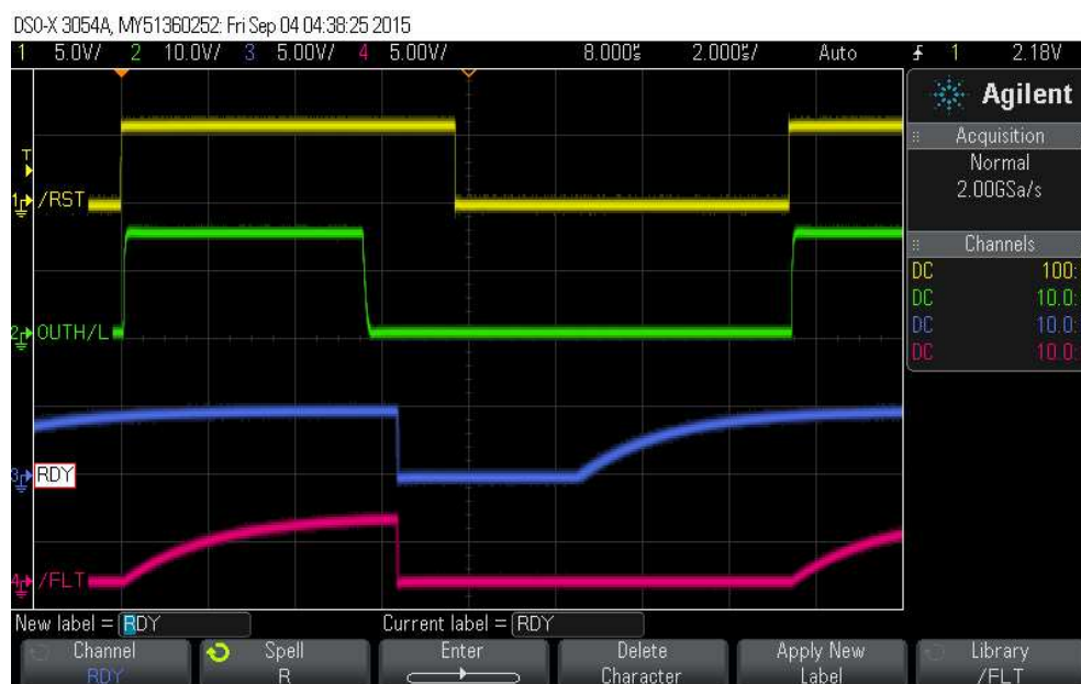
Figure 7. ISO5852S EVM OUTH/L, RDY, \overline{\text{FLT}} , and \overline{\text{RST}} With Unipolar Output Supply
