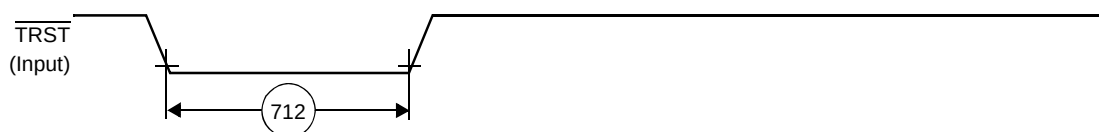
Figure 25. \overline{\text{TRST}} Timing Diagram
