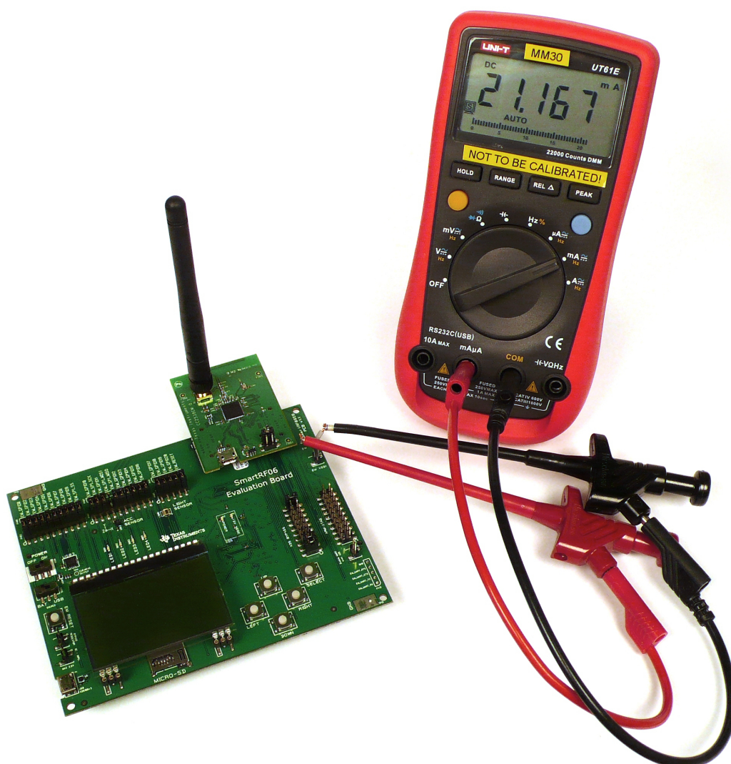
Figure 23. Measuring Current Consumption Using Jumper J503
