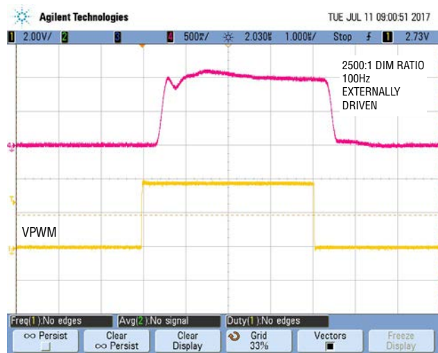
Figure 3. High Performance PWM Dimming with (a) Internally Generated PWM Dimming and (b) Externally Driven PWM Dimming
