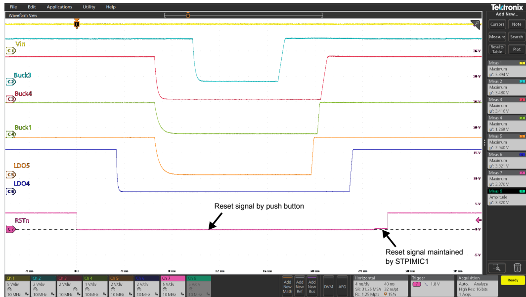
Figure 13. Reset sequence for STPMIC1A configuration
