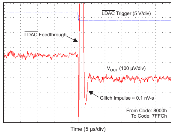
Figure 82. Glitch Impulse, Falling Edge, 4-LSB Step
