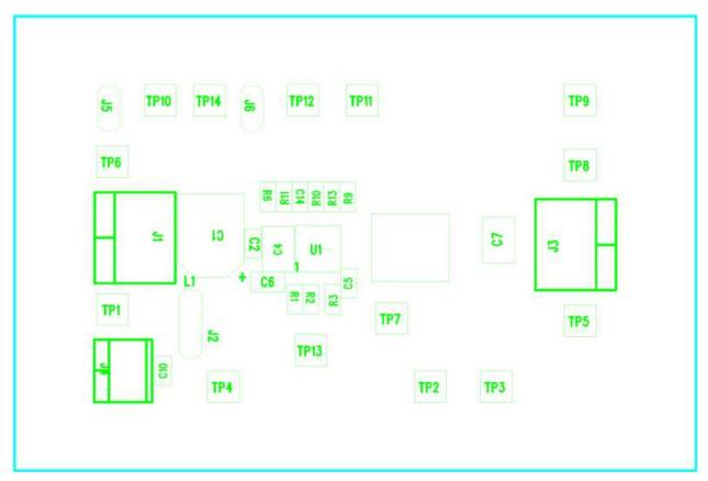
Figure 16. TPS54020EVM-082 Top Side Component Placement
