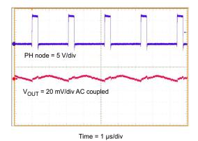
Figure 6. TPS54020EVM-082 Output Ripple
