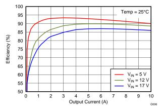
Figure 1. EVM Efficiency at 25°C
