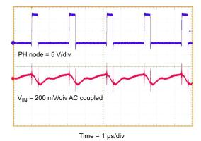
Figure 7. TPS54020EVM-082 Input Ripple
