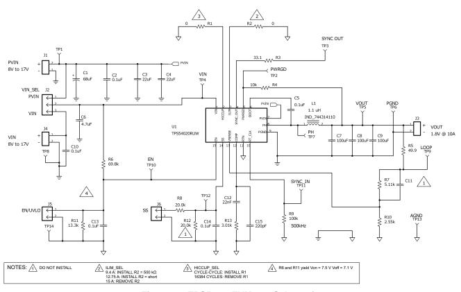
Figure 18. TPS54020EVM-082 Schematic
