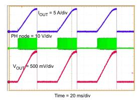
Figure 11. TPS54020EVM-082 Hiccup Mode Current Limit
