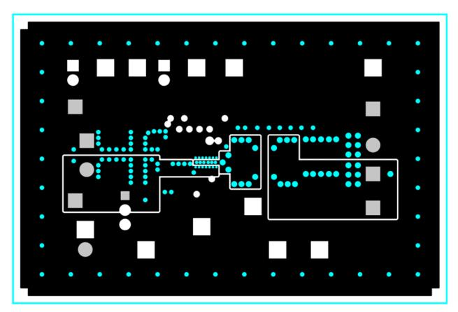
Figure 13. TPS54020EVM-082 Internal 1 Copper
