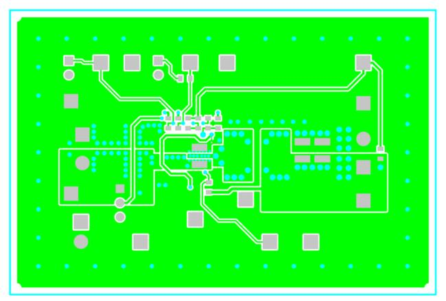
Figure 15. TPS54020EVM-082 Bottom Side Copper
