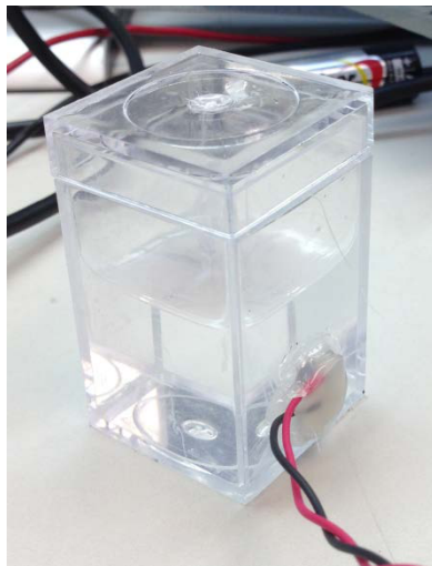
Figure 2. Water Container with 1-MHz Transducer
