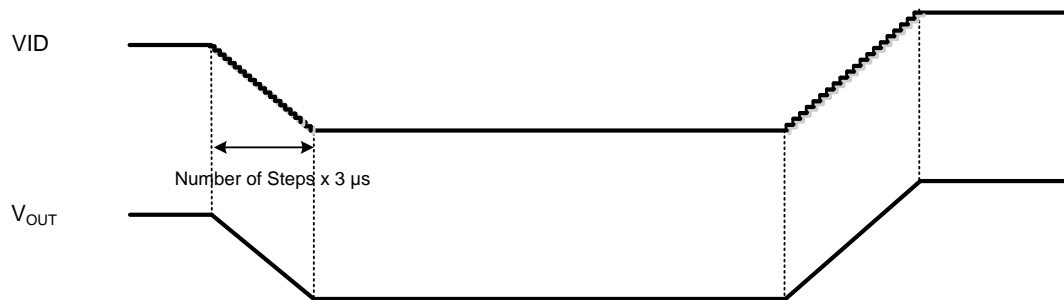
Figure 5-4. DVS Timing Diagram I (BUCKx_DECAY = 0)
