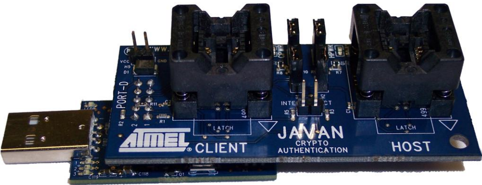
Figure 1-2. The AT88CK109BK8 adaptor board with the Atmel AT88Microbase
