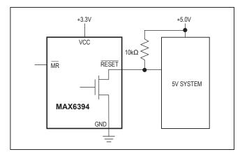
Figure 1. MAX6394 Open-Drain RESET Output Allows Use with Multiple Supplies
