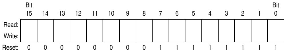
Figure 7-4. Stack Pointer (SP)
