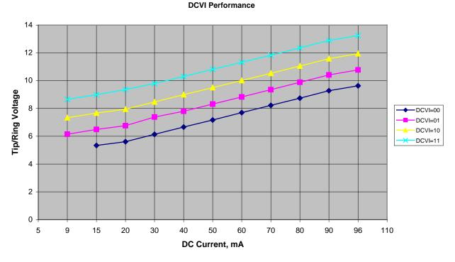
Figure 2: DC Line Characteristics with the 73M1x22 DCVI(1:0) Settings
