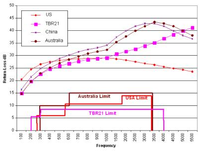
Figure 1: 73M1x22 Return Loss Characteristics
