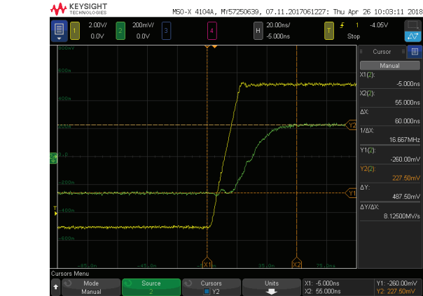
Figure 9. The settling time of the LT6275 (CH1-Input, CH2-Output).
