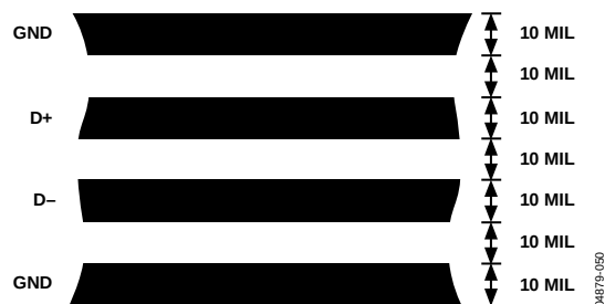
Figure 50. Arrangement of Signal Tracks
