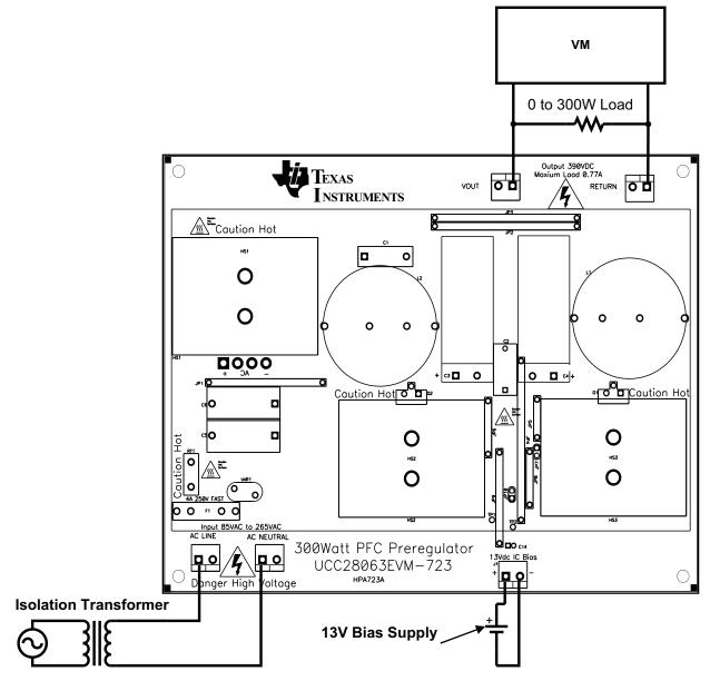
Figure 3. Test Setup
