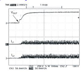
Figure 15. Start-Up at  $V_{IN} = 85 V_{RMS}$ ,  $P_{OUT} = 300 W$
