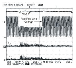
Figure 19. Line Transient,  $P_{OUT} = 300W$
