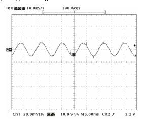
Figure 8.  $V_{OUT}$  Ripple,  $P_{OUT} = 300 \text{ W}$
