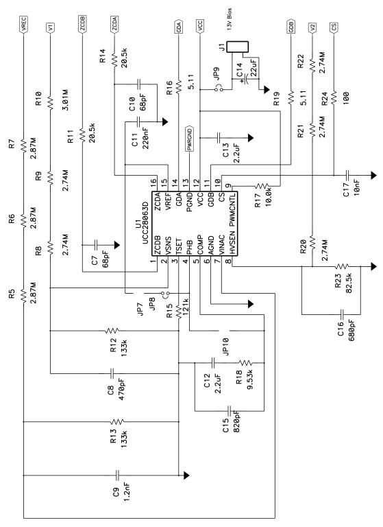
Figure 2. Controller Circuitry
