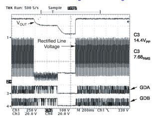
Figure 18. Brownout at 265 V<sub>RMS</sub>
