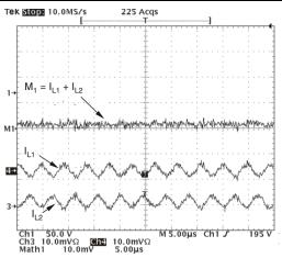
Figure 12. Inductor and Input Ripple Current at 265  $V_{\text{RMS}}$  Input at Half Peak Line Voltage
