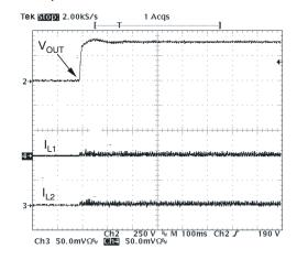
Figure 16. Start-Up at  $V_{IN} = 265 V_{RMS}$ ,  $P_{OUT} = 0 W$
