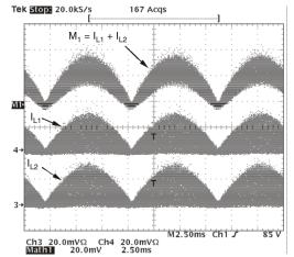
Figure 13. Inductor and Input Ripple Current at  $V_{IN}$  = 85  $V_{RMS}$ ,  $P_{OUT}$  = 300 W
