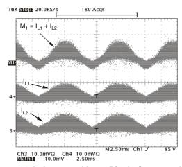
Figure 14. Inductor and Input Ripple Current at  $\rm V_{IN} = 265~V_{RMS},~P_{OUT} = 300~W$
