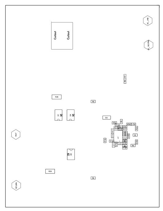
Figure 22. Bottom Layer Assembly
