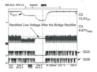
Figure 17. Brownout at 85 V<sub>RMS</sub>
