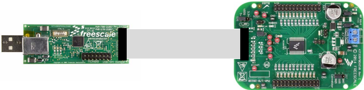
Figure 6. Connecting KITUSBSPIDGLEVME to the Evaluation Board
