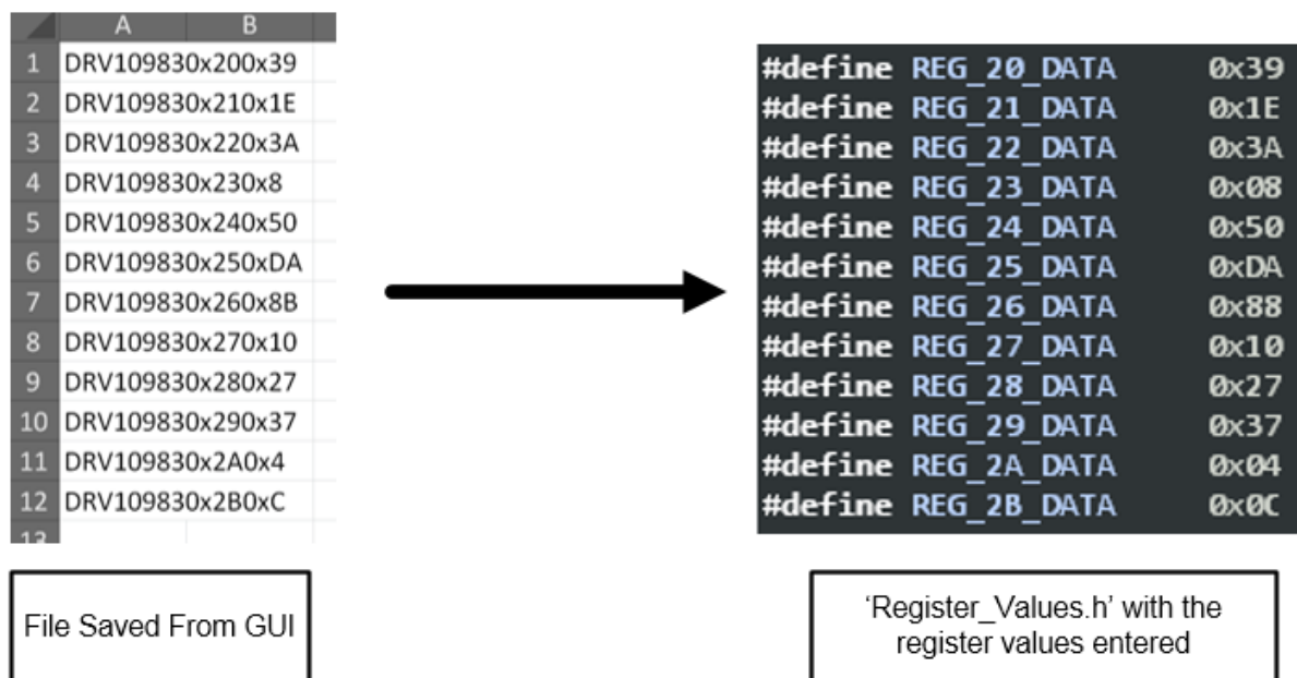
Figure 18. Example Register Settings Entered into the Programming Tools Code for DRV10983
