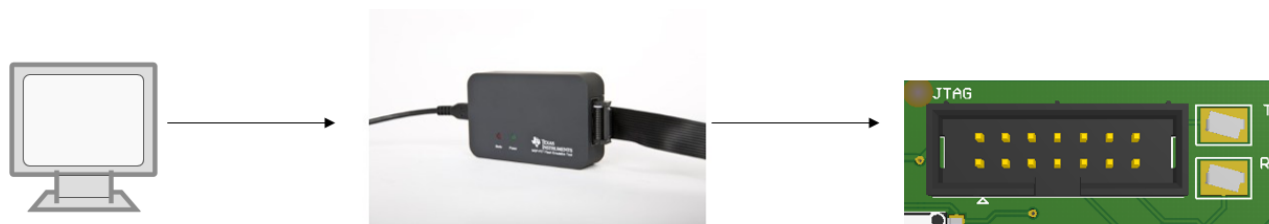
Figure 19. MSP-FET and TIDA-01373 System Diagram
