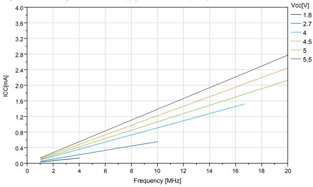
Figure 33-54. ATmega324PB: Reset Supply Current vs.  $V_{cc}$  (Excluding current through Reset Pullup)
