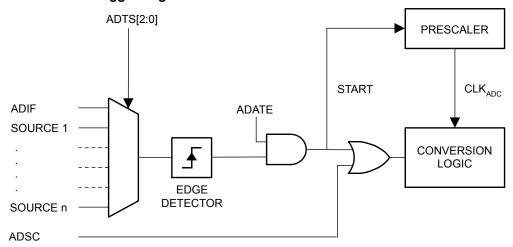
Using the ADC Interrupt Flag as a trigger source makes the ADC start a new conversion as soon as the ongoing conversion has finished. The ADC then operates in Free Running mode, constantly sampling and updating the ADC Data Register. The first conversion must be started by writing a '1' to ADCSRA.ADSC. In this mode the ADC will perform successive conversions independently of whether the ADC Interrupt Flag (ADIF) is cleared or not.
