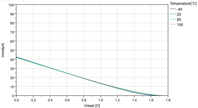
Figure 33-20. ATmega324PB: Reset Pull-up Resistor Current vs. Reset Pin Voltage ( $V_{CC}$  = 2.7V)
