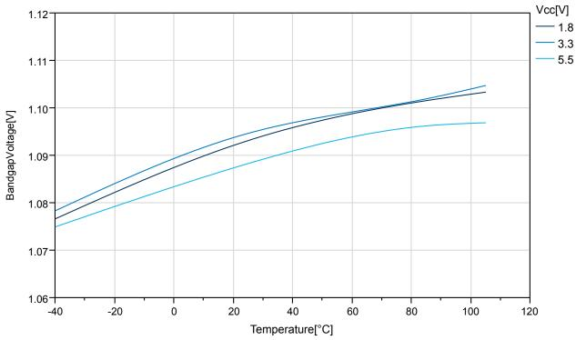
Figure 33-36. ATmega324PB: Calibrated Bandgap Voltage vs.  $V_{cc}$
