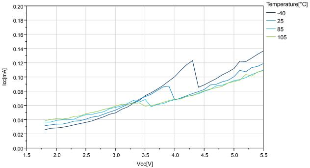
Figure 33-50. ATmega324PB: AREF External Reference Current vs.  $V_{\rm cc}$
