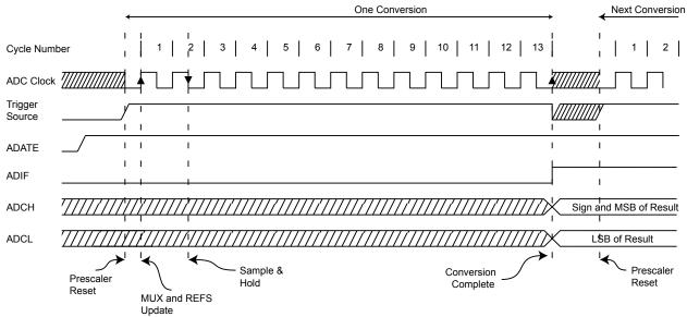
Figure 27-7. ADC Timing Diagram, Free Running Conversion
