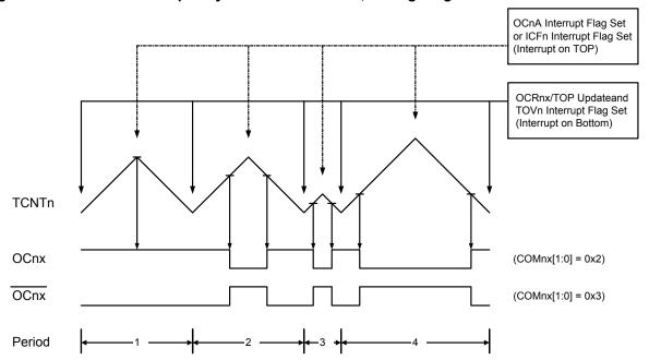
**Note:** The "n" in the register and bit names indicates the device number (n = 1, 3, 4 for Timer/Counter 1, 3, 4), and the "x" indicates Output Compare unit (A/B).
