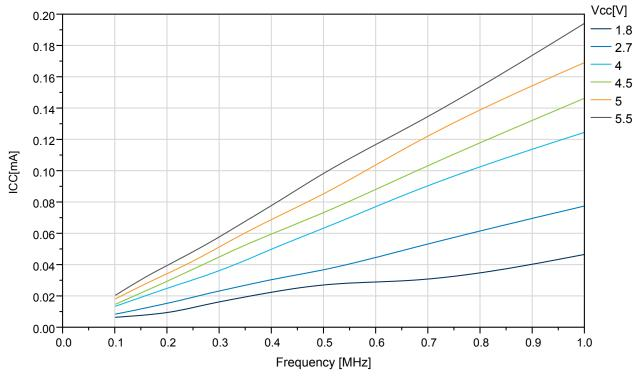
Figure 33-9. ATmega324PB: Idle Supply Current vs. Frequency (1-20MHz)
