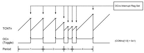
An interrupt can be generated each time the counter value reaches the TOP value by setting the OCF0A Flag. If the interrupt is enabled, the interrupt handler routine can be used for updating the TOP value.
