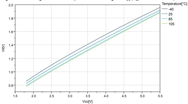
Figure 33-28. ATmega324PB I/O Pin Input Hysteresis vs. VCC
