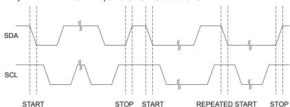
Figure 25-3. START, REPEATED START, and STOP conditions
