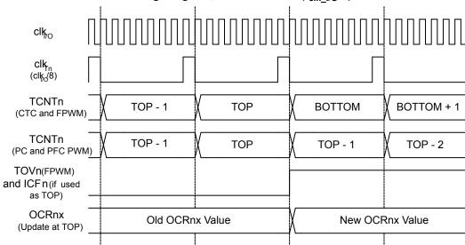
Figure 18-12. Timer/Counter Timing Diagram, with Prescaler (f<sub>clk I/O</sub>/8)
