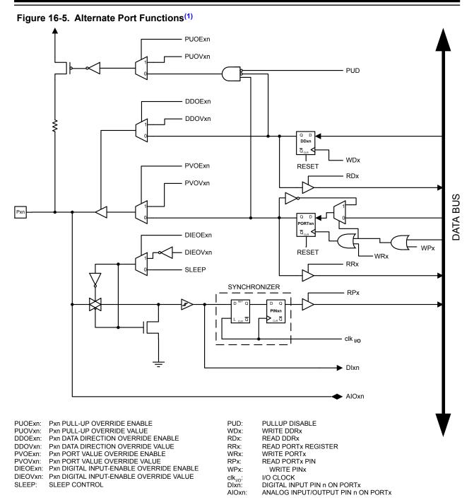
**Note:** 1. WRx, WPx, WDx, RRx, RPx, and RDx are common to all pins within the same port.  $clk_{I/O}$ , SLEEP, and PUD are common to all ports. All other signals are unique for each pin.
