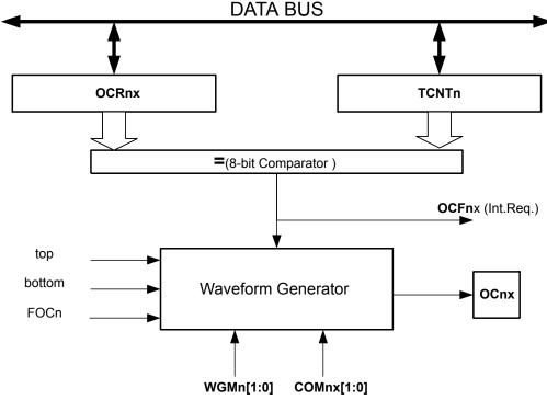
**Note:** The "n" in the register and bit names indicates the device number (n = 0 for Timer/Counter 0), and the "x" indicates Output Compare unit (A/B).
