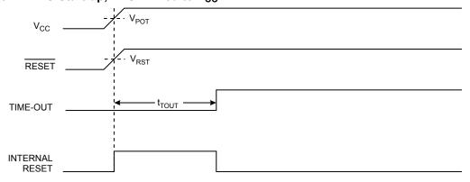
Figure 13-3. MCU Start-up, RESET Extended Externally
