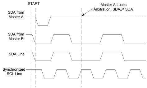
Figure 25-8. Arbitration Between Two Masters
