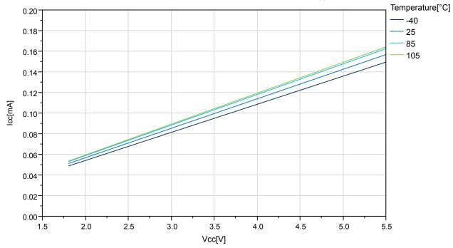
Figure 33-51. ATmega324PB: Programming Current vs. V<sub>cc</sub>
