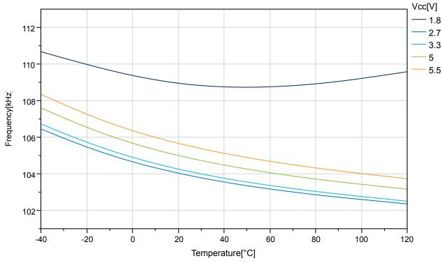
Figure 33-42. ATmega324PB: Watchdog Oscillator Frequency vs.  $V_{CC}$
