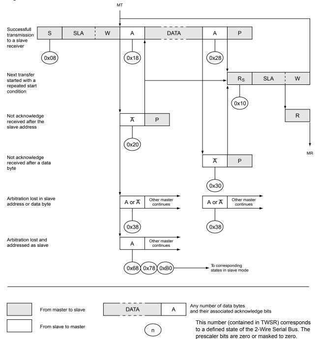
Figure 25-12. Formats and States in the Master Transmitter Mode
