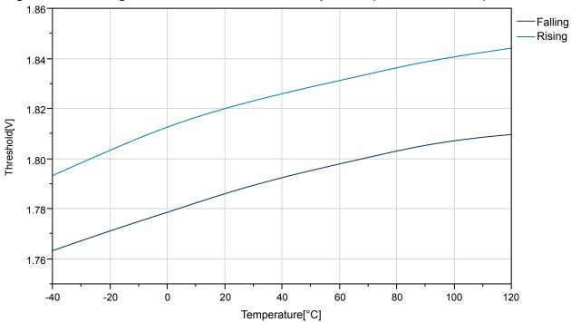
Figure 33-33. ATmega324PB: BOD Thresholds vs. Temperature (BODLEVEL is 2.7V)
