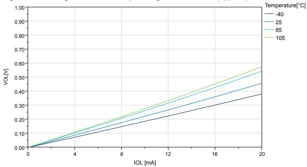
Figure 33-24. ATmega324PB: I/O Pin Output Voltage vs. Source Current ( $V_{CC} = 3V$ )
