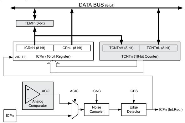
Figure 18-2. Input Capture Unit Block Diagram for TCn
