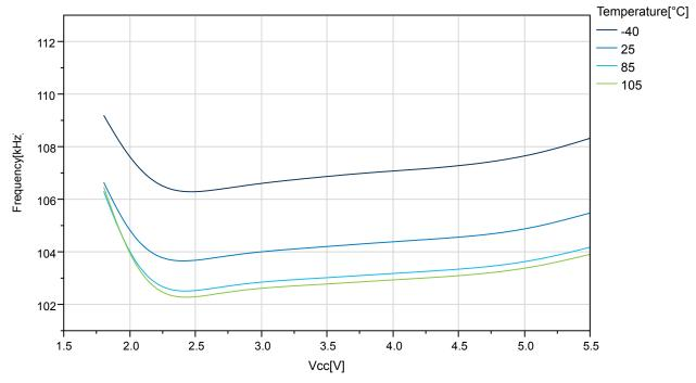
Figure 33-43. ATmega324PB: Calibrated 8MHz RC Oscillator Frequency vs.  $V_{\text{CC}}$
