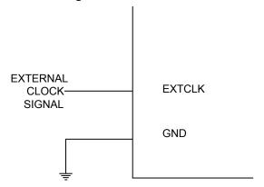
When this clock source is selected, start-up times are determined by the SUT Fuses:
