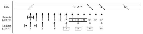
The same majority voting is done to the stop bit as done for the other bits in the frame. If the stop bit is registered to have a logic '0' value, the Frame Error (UCSRnA.FE) Flag will be set.
