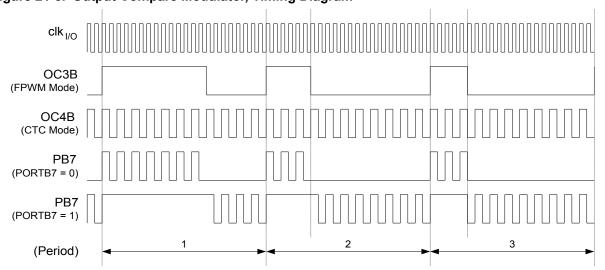
Figure 21-3. Output Compare Modulator, Timing Diagram
