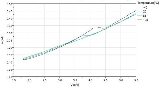
Figure 33-48. ATmega324PB: ADC Current vs.  $V_{cc}$  (AREF =  $AV_{cc}$ ), No Conversion Temperature[°C] -40 0.45 25 85 0.40 105 0.35 0.30 [cc[mA] 0.25 0.20 0.15 0.10 0.05 0.00 2.0 2.5 3.0 3.5 5.0 4.0 4.5 5.5 1.5
