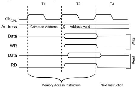
Figure 9-3. On-chip Data SRAM Access Cycles
