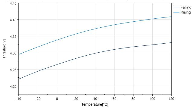
Figure 33-35. ATmega324PB: Calibrated Bandgap Voltage vs. Temperature
