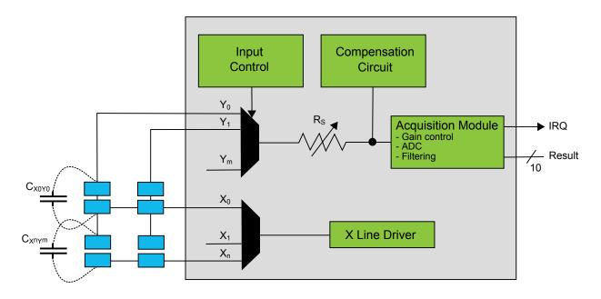
Figure 28-2. PTC Block Diagram Self-Capacitance
