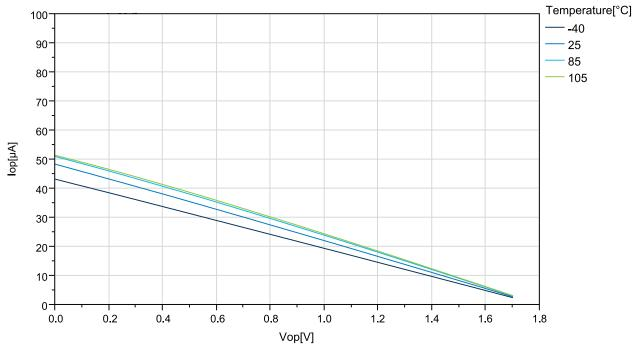
Figure 33-17. ATmega324PB: I/O Pin Pull-up Resistor Current vs. Input Voltage (V<sub>CC</sub> = 2.7V)
