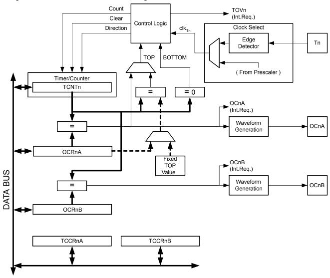
Figure 20-1. 8-bit Timer/Counter Block Diagram
