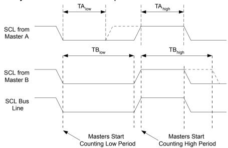
Figure 25-7. SCL Synchronization Between Multiple Masters
