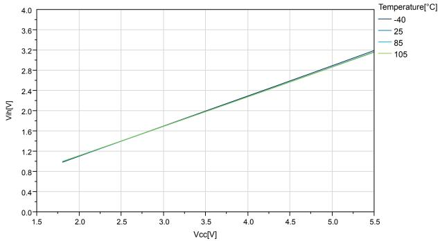
Figure 33-27. ATmega324PB I/O Pin Input Threshold Voltage vs. V<sub>CC</sub> (V<sub>IL</sub>, I/O Pin read as '0')
