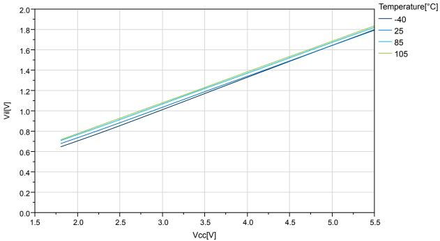
Figure 33-31. ATmega324PB Reset Pin Input Hysteresis vs. VCC
