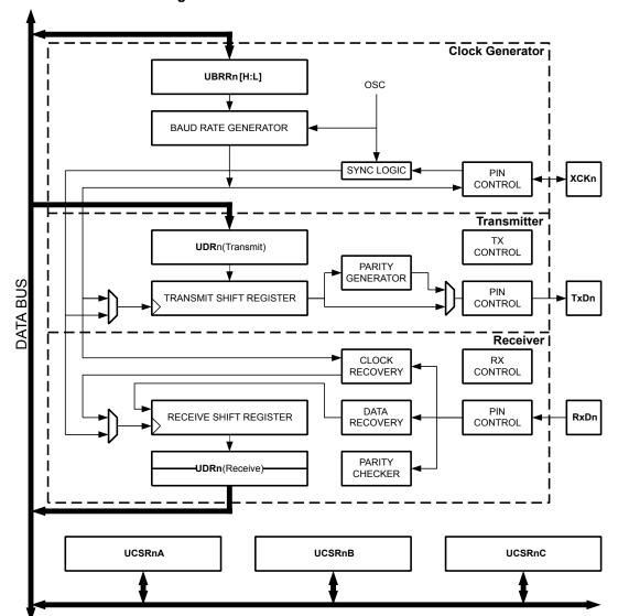
Figure 23-1. USART Block Diagram
