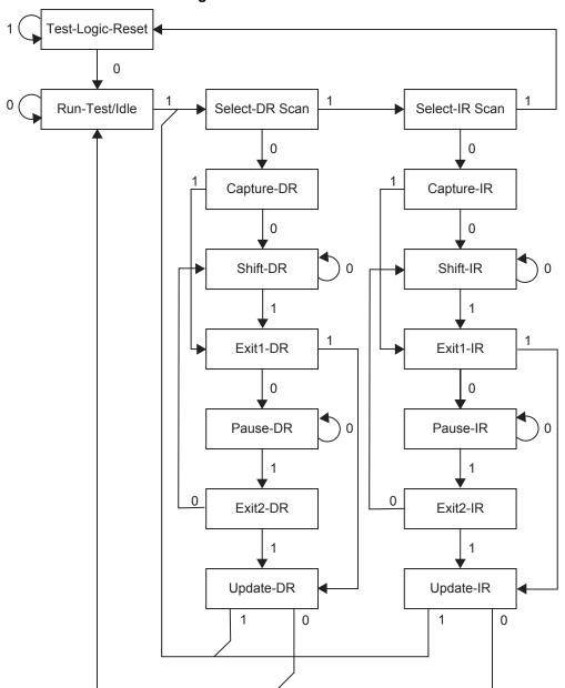
Figure 29-2. TAP Controller State Diagram
