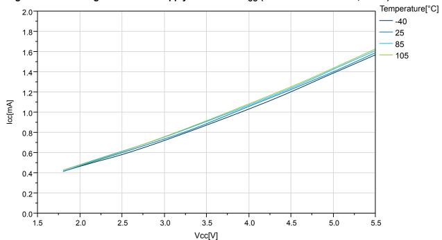
Figure 33-12. ATmega324PB: Idle Supply Current vs. V<sub>CC</sub> (Internal RC Oscillator, 8MHz)
