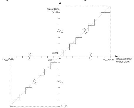
Figure 27-14. Differential Measurement Range
