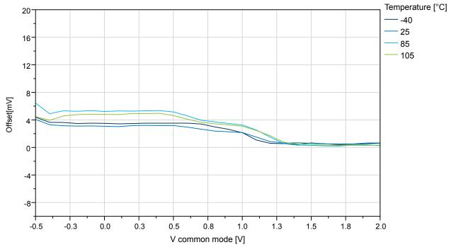
Figure 33-39. ATmega324PB: AC Offset vs. Common Voltage (V<sub>CC</sub> = 3.0V)
