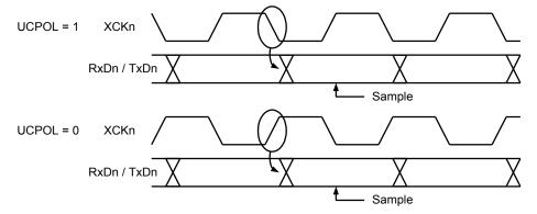
The UCPOL bit UCRSC selects which XCKn clock edge is used for data sampling and which is used for data change. As the above timing diagram shows, when UCPOL is zero, the data will be changed at rising XCKn edge and sampled at falling XCKn edge. If UCPOL is set, the data will be changed at falling XCKn edge and sampled at rising XCKn edge.
