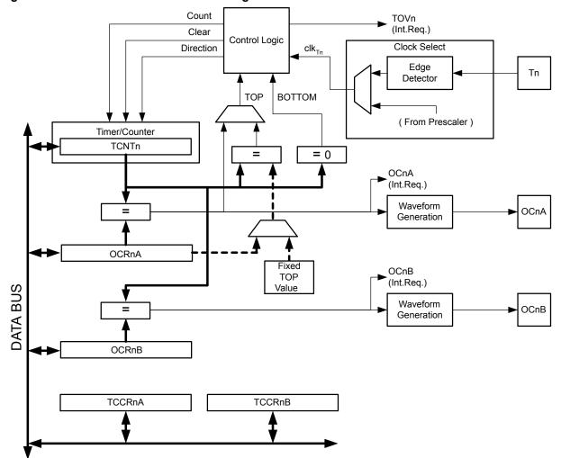
Figure 17-1. 8-bit Timer/Counter Block Diagram
