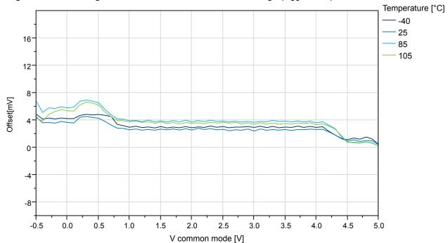
Figure 33-40. ATmega324PB: AC Offset vs. Common Voltage (V<sub>CC</sub> = 5.0V)
