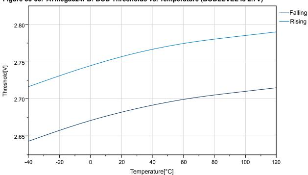
Figure 33-34. ATmega324PB: BOD Thresholds vs. Temperature (BODLEVEL is 4.3V)
