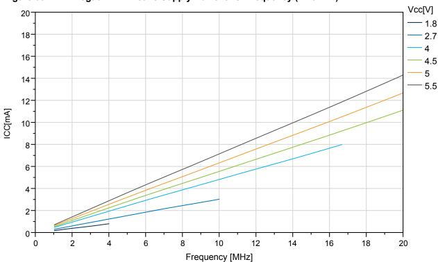
Figure 33-2. ATmega324PB: Active Supply Current vs. Frequency (1-20MHz)
