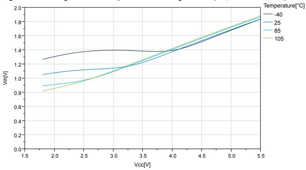
Figure 33-30. ATmega324PB Reset Input Threshold Voltage vs. VCC (VIL, I/O Pin read as '0')
